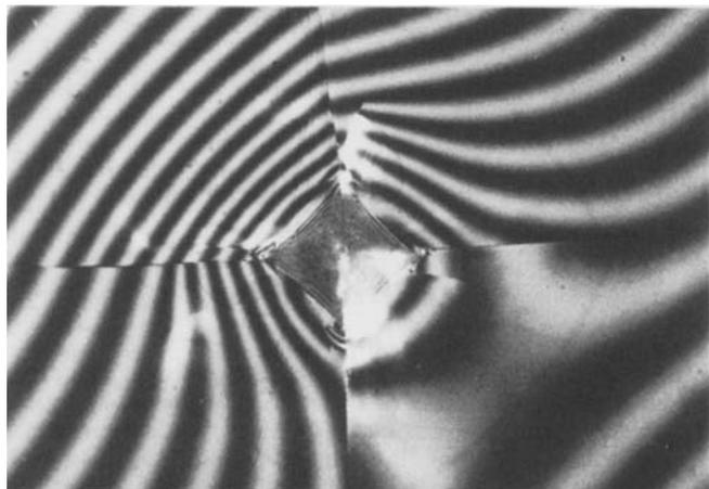
Fig. 2. Vickers indentation ( $P=50$  N) in soda-lime glass; interference fringe micrograph, sodium light. Fringe distortion indicates surface uplift of material above lateral crack plane. Note distortion contained within bounds of radial crack traces (width of micrograph= $625 \mu\text{m}$ ).
